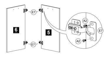
Assemble the Hinges 2/8 (E7) at panel no. 7 & 8 by using Screw m3.5 x 14mm (A2). STEP 6
