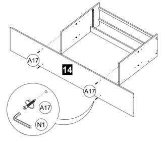
STEP 15 Assemble the panel no. 1 & 2 by using Crosshead Screw m6.3 x 40mm (A17). Use Allen Key (N1) to tighten the Crosshead Screw m6.3 x 40mm (A17) & button the screw head by using Crosshead Cover (Y).
