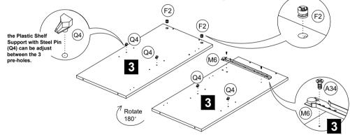
Insert the Plastic Shelf Support with Steel Pin (Q4) & Mini Fix Cam (F2) at panel no. 4. STEP 3 Assemble the Drawer Metal Slide 350mm (M6) at marking hole panel no. 4.
