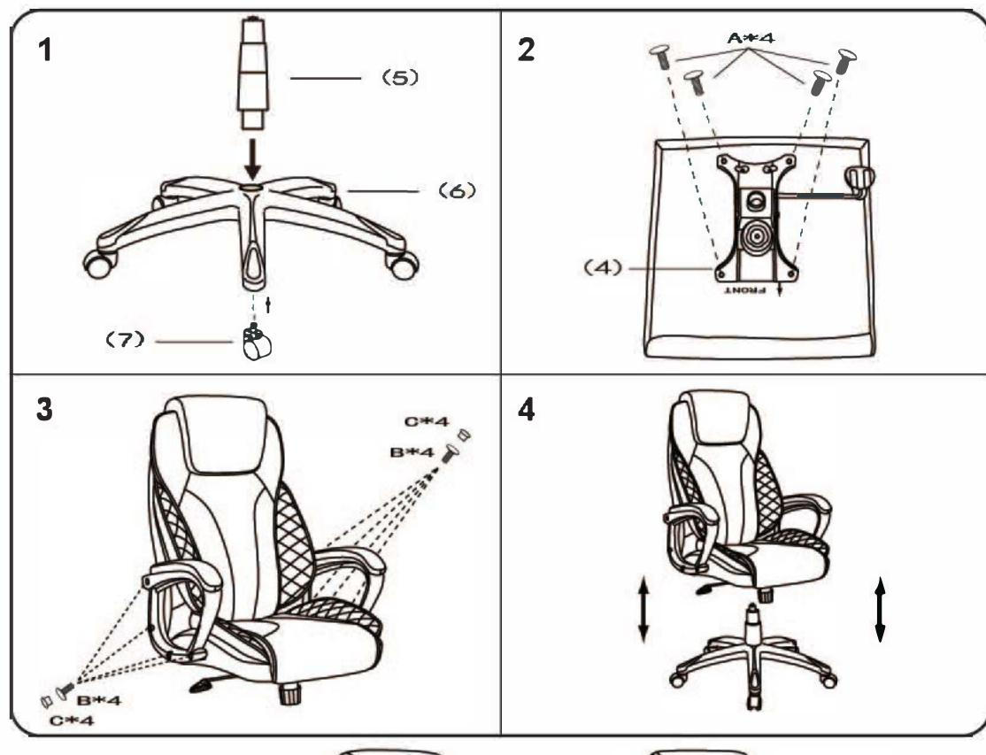
It is important to assemble all parts so that the directional "Arrows" point in the same direction.Make certain that all screws are FULLY tightened before using the chair.Each month, check all screws and tighten any that may have loosened
